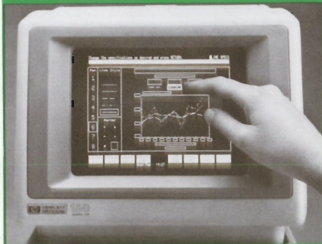
Textures and colors of graphs are changed by touching the HP 150's screen.
